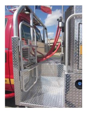
Two (2) 1" x 8 feet long 300# working pressure hose whips with threaded couplings shall be installed at front of body, one each side, with securement devices.
