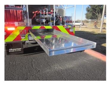
The rear center compartment shall be equipped with an .190" aluminum slide out tray on UHMW plastic slide pads. The tray shall be full width and full length of the compartment interior.
