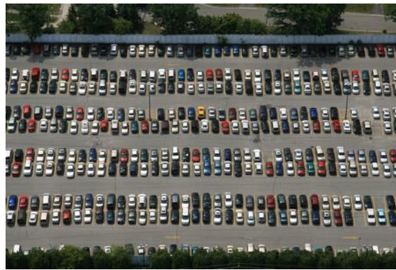
Demonstrates a parking lot with landscaping only on the perimeter of the lot
