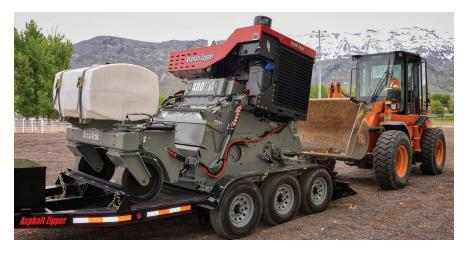
**Custom tandem-axle trailer** (optional) with quick-load guiding system, low center of gravity, convenient working deck and built-in custom toolbox, enables the 480Xi WA to be hauled behind a 1-ton pickup truck.
